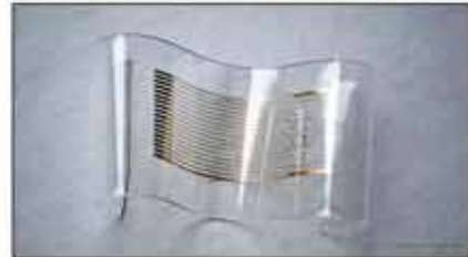
Schematic top-view of a microelectrode array being stretched along its length.
